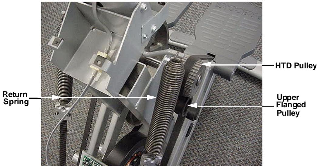
2. Support the stairarm and remove the stairarm belt from both flanged pulleys and the HTD pulley.
