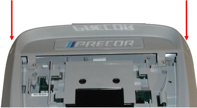
12. Remove the 6 screws that fasten the rear cover from the console and remove. **See Diagram 5.5.7.**
