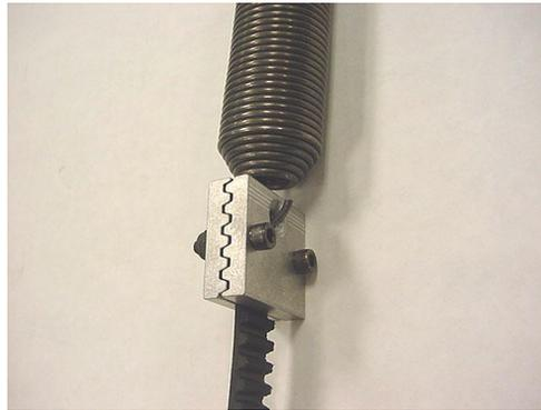
5. Remove the return spring from the other belt clamp. Remove the bolts that fasten the belt clamp to the belt and remove the belt from the clamp.
